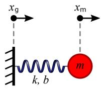
For the mass-spring system above, there is a restoring force proportional to the compression of the spring and a damping term proportional to the rate of change of the compression of the spring (assuming standard 'velocity' damping). We define the compression of the spring as the difference between ground and mass:
